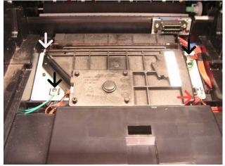
Remove Feed Roll by rotating roll opposite normal feed direction so release tabs are accessible, pushing in both release tabs, pulling top of roll away form shaft, rotating it down and disengaging lower mounting tabs.
