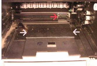
Remove LSU by disconnecting left electrical plug, removing Screws (3) and lifting LSU enough to access and disconnect right side electrical plug (CAUTION: Hold small PWB while disconnecting plug, red arrow).
