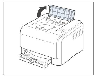
4. Holding the inner cover open, carefully take the jammed paper out of the printer. The inner cover will then close automatically.
