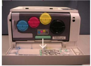
Remove InterTransfer Belt Unit by grasping bottom of ITB and pulling out slightly until it releases, lower it slightly, and continue pulling out to remove ITB. NOTE: Observe removal path for, especially rear of ITB for reinstallation. CAUTION: Do not touch the ITB Belt. Protect it from light.
