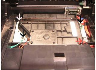
4. Remove Tray Empty Actuator by removing Screw and pulling Actuator housing up. NOTE: a small locating tab on the bottom, under arrow, will resist upward movement while disengaging.
