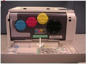
2. Remove InterTransfer Belt Unit by grasping bottom of ITB and pulling out slightly until it releases, lower it slightly, and continue pulling out to remove ITB. NOTE: Carefully observe removal path, especially at rear of ITB, for reinstallation. CAUTION: Do not touch the ITB Belt. Protect it from light.
