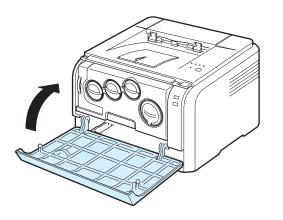
**CAUTION**: If the front cover is not completely closed, the printer will not operate.
