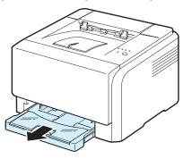
**2** Pressing and unlatching the guide lock in the top of the tray, pull the tray out manually.
