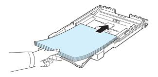
Make sure not to overfill the tray and that all four corners are flat in the tray and under the brackets, as shown below. Overfilling the tray may cause a paper jam.
