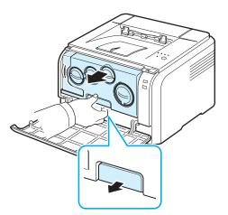
4 Extend the top handle on the imaging unit and then use it to pull the imaging unit out of the printer completely.
