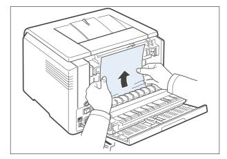
If you cannot find the jammed paper, or if there is any resistance removing the paper, stop pulling and go to the next step.
