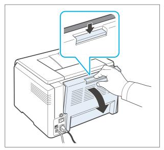
2. Carefully remove the paper by pulling in the direction as shown below. Most of the jammed paper can be removed in this step.
