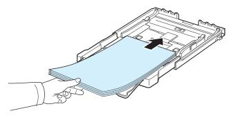
4 Slide the paper length guide until it lightly touches the end of the paper stack. Squeeze the paper width guide and slide it to the edge of the paper stack without causing it to bend.
