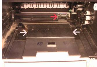
3. Remove LSU by disconnecting left electrical plug, removing Screws (3) and lifting LSU enough to access and disconnect right side electrical plug (CAUTION: Hold small PWB while disconnecting plug, red arrow).
