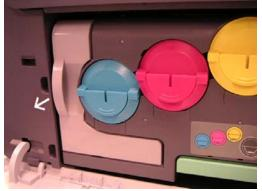
2. Remove the Waste Toner Retainer Cap from the storage position and install the cap on the return port. Secure the Waste Toner Cartridge into the top of the machine for shipping.
