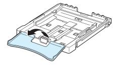
**3** Unlatch the tray locks in the middle of the tray by pressing them firmly and pull the tray out to extend it.
