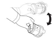
4 Remove the cartridges cap.
