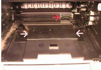
3. Disconnect left electrical plug, remove Screws (3) and lift LSU enough to access and disconnect right side electrical plug and remove LSU.
