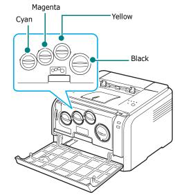
**6** Grasp the toner cartridges and align them with the slots inside the printer. Insert them into their corresponding slots until they click into place.
