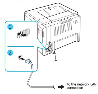
**3** Plug the other end of the cable into a network LAN connection.
